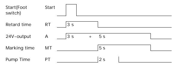
The display shows what is happening at the moment. For example, when the retard time is activated, the display will switch from marking time (MT) to retard time (RT).
