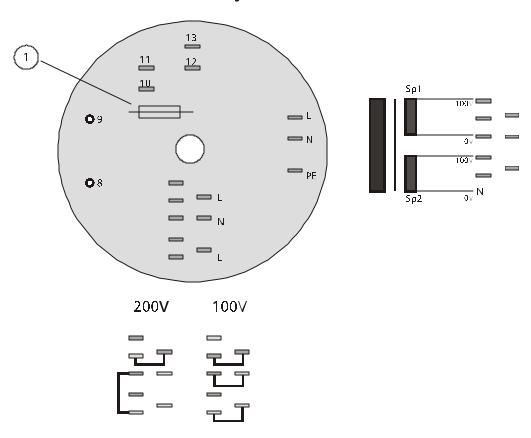
The bridges available enable the following input voltages (see drawing): 100 V or 200 V.
