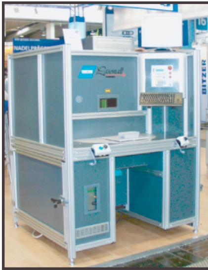
The Lasonall RT 800 is a fully automatic Class I laser marking system. It features an 800 mm indexing rotary table, an integrated automatic z-axis, integral interlocking, and a safety viewing glass. The system is ideal for production environments requiring an automated and fast marking system that is easy to use and safe.
